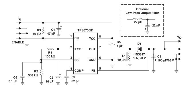
Figure 15. Application Circuit
