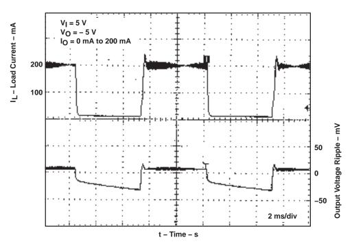
**Figure 4. Load Transient Response**
