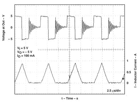
Figure 2. Switching Waveforms
