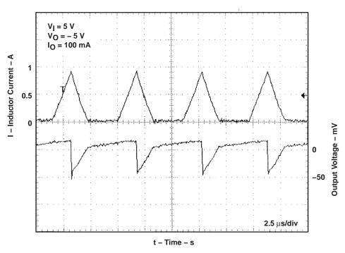
Figure 3. Output Voltage Ripple
