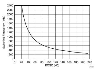
Figure 30. ROSC vs Switching Frequency
