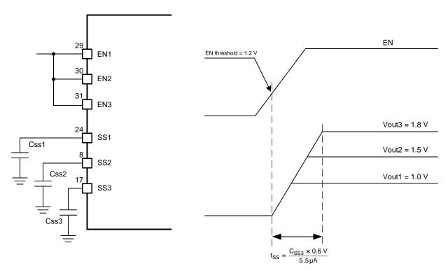
Figure 26. Simultaneous Startup Sequence Using SSx Pins
