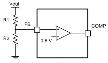
Figure 21. Voltage Divider Circuit
