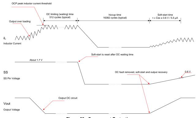
Figure 29. Overcurrent Protection
