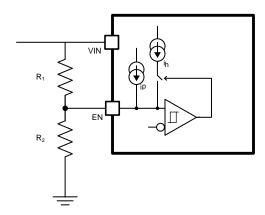
Figure 23. Adjustable VIN UVLO, VINQ > 2.7 V
