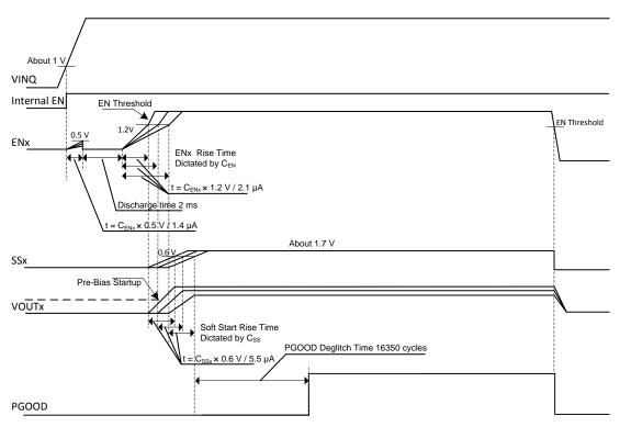
Figure 27. Startup Power Sequence
