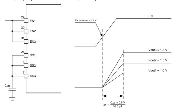
Figure 25. Ratiometric Power-Up Using SSx Pins
