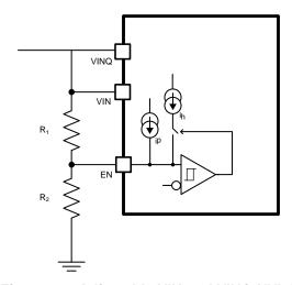
Figure 24. Adjustable VIN and VINQ UVLO
