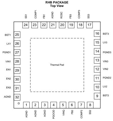
A. There is no electric signal down bonded to thermal pad inside IC. Exposed thermal pad must be soldered to PCB for optimal thermal performance.
