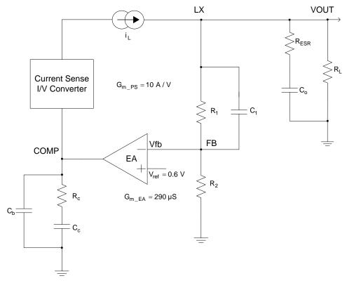
Figure 33. DC/DC Loop Compensation
