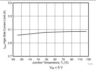
Figure 19. Buck2 High-Side Current Limit vs Temperature
