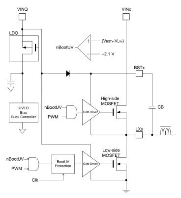
Figure 28. Bootstrap Voltage and Diagram
