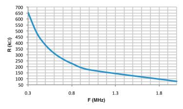
Figure 13. ROSC vs Switching Frequency
