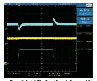
Figure 12. Buck 2 (Blue Trace) Dynamic Response 0.5-A - 1.5-A Step, 50 mV/div. Buck 1 (Yellow Trace), 50 mV/div  $V_{\text{IN}}$  = 12 V, f<sub>SW</sub> = 500 kHz, L<sub>O</sub> = 4.7 µH, DCR = 10 m $\Omega$ , C<sub>O</sub> = 22 µF
