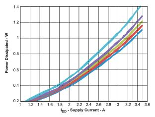
Figure 21. Buck 1  $V_{IN}$  = 12 V,  $f_S$  = 500 kHz,  $V_O$  (From Top to Bottom) = 5, 3.3, 2.5, 1.8, 1.2 V
