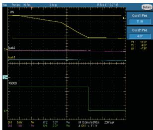
Figure 9. Power Down Behavior (From Top to Bottom  $V_{IN}$ , Buck2 = 1.8 V, Buck1 = 1.2 V, PGOOD)  $V_{IN} = 12 \text{ V, } f_{SW} = 500 \text{ kHz, } L_O = 4.7 \text{ } \mu\text{H,} \\ DCR = 10 \text{ } m\Omega, C_O = 22 \text{ } \mu\text{F}$
