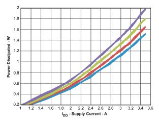
Figure 26. Buck 2  $V_{\rm IN}$  = 5 V,  $f_{\rm S}$  = 500 kHz,  $V_{\rm O}$  (From Top to Bottom) = 5, 3.3, 2.5, 1.8, 1.2 V
