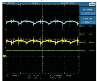
Figure 10. Ripple for Buck 1 (Yellow Trace) 1.2 V, 3 A and Buck 2 (Blue Trace) 1.8 V, 2 A, 50 mV per Division  $V_{\text{IN}}$  = 12 V,  $f_{\text{SW}}$  = 500 kHz,  $L_{\text{O}}$  = 4.7  $\mu\text{H}$ , DCR = 10 m $\Omega$ ,  $C_{\text{O}}$  = 22  $\mu\text{F}$
