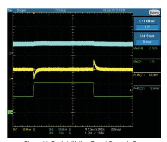
Figure 11. Buck 1 (Yellow Trace) Dynamic Response 1-A - 2-A Step, 50 mV/div. Buck 2 (Blue Trace), 50 mV/div  $V_{IN}$  = 12 V,  $f_{SW}$  = 500 kHz,  $L_O$  = 4.7  $\mu$ H, DCR = 10 m $\Omega$ ,  $C_O$  = 22  $\mu$ F
