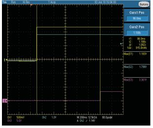
Figure 8. Power Up and PGOOD (From Top to Bottom, Buck2 = 1.8 V, Buck1 = 1.2 V, PGOOD)  $V_{IN} = 12~V, f_{SW} = 500~kHz, L_O = 4.7~\mu H, \\ DCR = 10~m\Omega, C_O = 22~\mu F$
