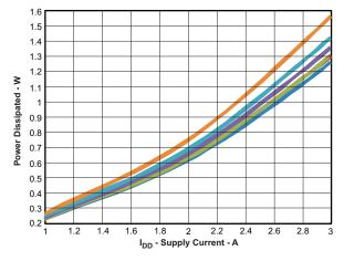
Figure 22. Buck 2  $V_{IN}$  = 12 V,  $f_S$  = 500 kHz,  $V_O$  (From Top to Bottom) = 5, 3.3, 2.5, 1.8, 1.2 V
