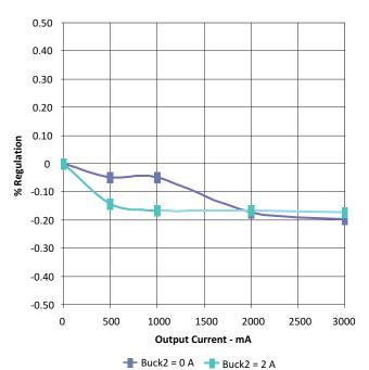
Figure 1. Buck1 Load Regulation, Vo = 1.2 V
