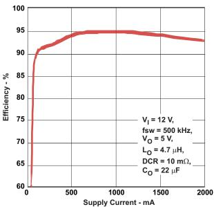
Figure 5. Buck 2 Efficiency,  $V_O$  = 5 V,  $V_{IN}$  = 12 V,  $f_{SW}$  = 500 kHz,  $L_O$  = 4.7  $\mu$ H, DCR = 10 m $\Omega$ ,  $C_O$  = 22  $\mu$ F
