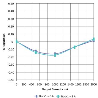
Figure 2. Buck2 Load Regulation V<sub>O</sub> = 1.8 V
