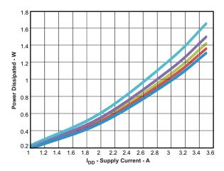
Figure 23. Buck 1  $V_{IN}$  = 12 V,  $f_S$  = 1.1 MHz,  $V_O$  (From Top to Bottom) = 5, 3.3, 2.5, 1.8, 1.2 V
