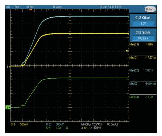
Figure 7. Soft Start for Buck 1 (Yellow Trace) 1.2 V, 3 A and Buck 2 (Blue Trace) 1.8 V, 2 A,  $V_{IN}=12\ V,\ f_{SW}=500\ kHz,\ L_O=4.7\ \mu H,\\ DCR=10\ m\Omega,\ C_O=22\ \mu F$
