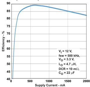
Figure 6. Buck 2 Efficiency,  $V_O$  = 3.3 V,  $V_{IN}$  = 12 V,  $f_{SW}$  = 500 kHz,  $L_O$  = 4.7  $\mu$ H, DCR = 10 m $\Omega$ ,  $C_O$  = 22  $\mu$ F
