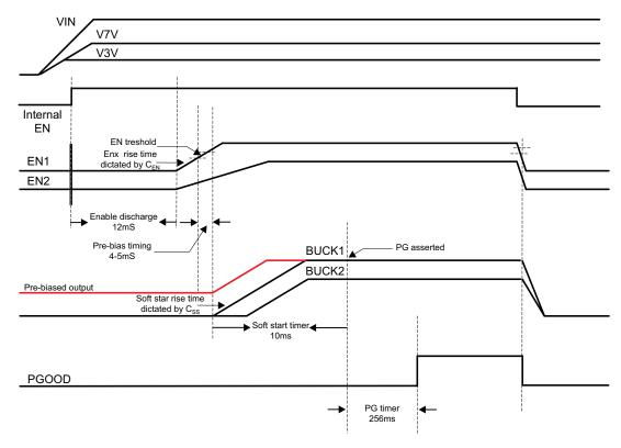
Figure 14. Start-Up Sequencing and PGOOD Signal Generation
