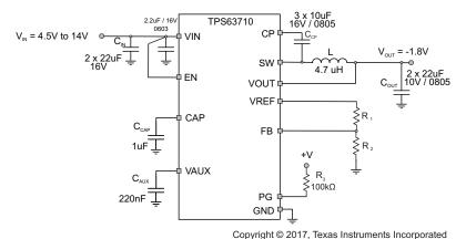
Figure 10. Typical Application for an Input Voltage up to 14V
