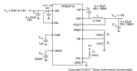
Figure 42. Typical Application for an Output Voltage of -5 V
