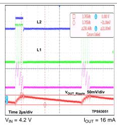
Figure 25. Output Voltage Ripple in Buck Mode and PFM to PWM Transition
