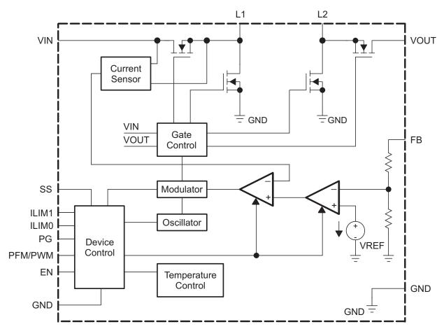
Figure 5. TPS63051 Block Diagram
