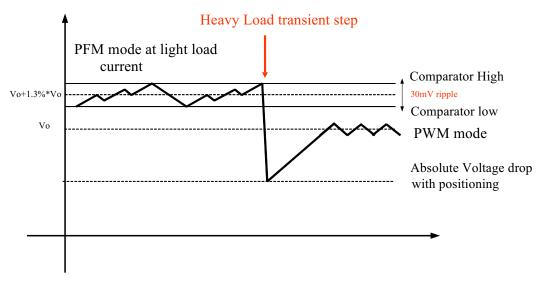
Figure 7. Power Save Mode Operation
