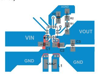
Figure 35. TPS6305x Layout (HotRod)
