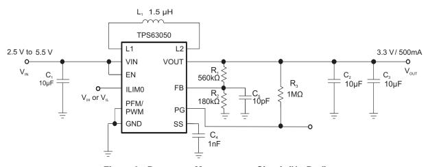
Figure 9. Parameter Measurement Circuit (HotRod)
