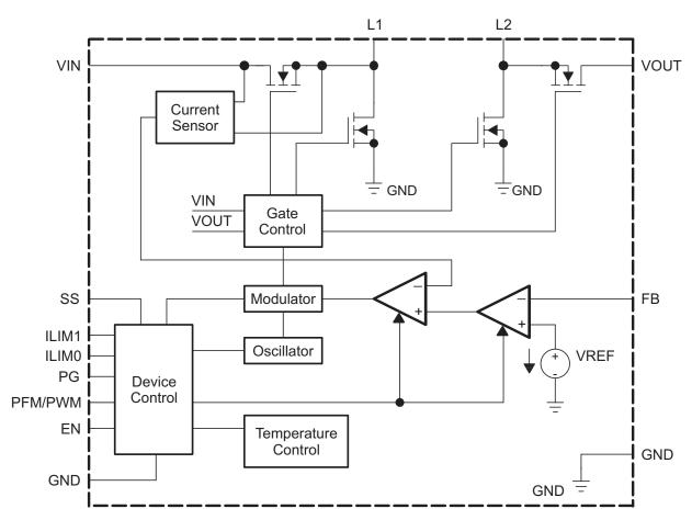
Figure 4. TPS63050 Block Diagram
