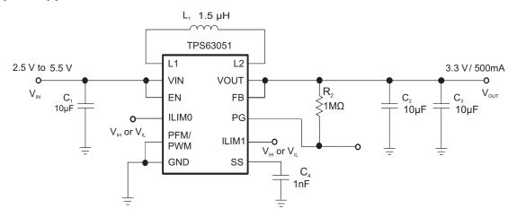
Figure 8. Parameter Measurement Circuit (WCSP)
