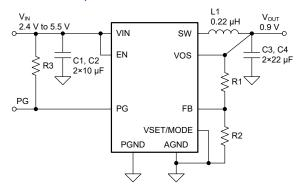
**Typical Application Schematics - Adjustable Output Voltage**
