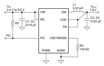
Figure 8-2. Fixed Start-up Output Voltage Application Circuit
