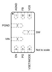
Figure 6-1. 9-Pin RQY QFN Package (Top View)
