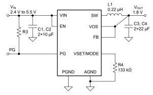
Typical Application Schematics - Fixed Output Voltage
