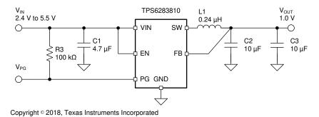
Figure 5. Typical Application of Fixed Output
