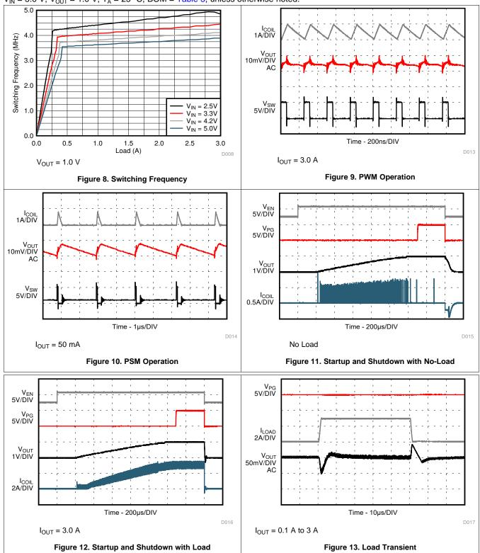
$V_{IN}$  = 5.0 V,  $V_{OUT}$  = 1.0 V,  $T_A$  = 25 °C, BOM = Table 3, unless otherwise noted.
