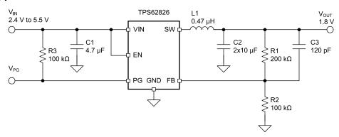
Figure 9-1. Typical Application of TPS62826x
