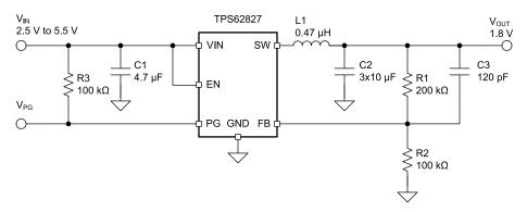
Figure 9-2. Typical Application of TPS62827
