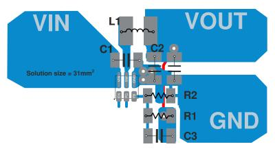
Figure 11-1. PCB Layout Recommendation
