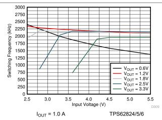
Figure 9-23. Switching Frequency
