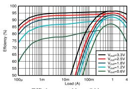
Efficiency at V<sub>IN</sub> = 5 V
