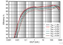
Efficiency Versus I<sub>OUT</sub> at 1.2 V<sub>OUT</sub>
