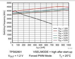
Figure 9-22. Switching Frequency vs Output Current
