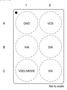
Figure 6-1. 6-Pin DSBGA YKA Package (Top View)
