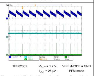
Figure 9-25. Typical Operation Power Save Mode
