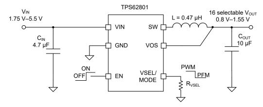
Figure 9-48. TPS62801 Adjustable V<sub>OUT</sub> Application Circuit
