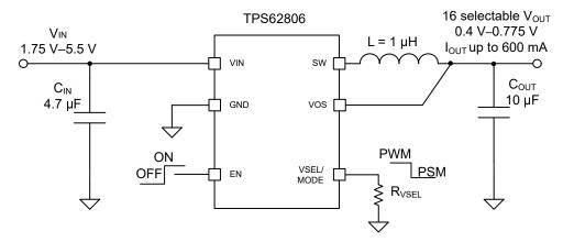
Figure 9-51. TPS62806 Adjustable V<sub>OUT</sub> Application Circuit
