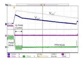
Figure 8-3. Optimized Transient Performance from PWM-to-PFM Mode
