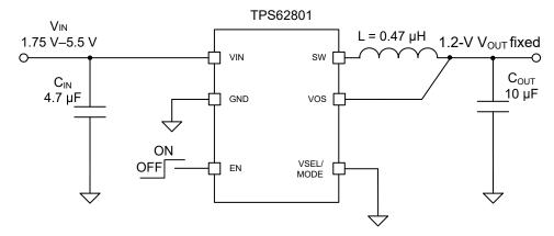
Figure 9-47. TPS62801 VSEL Connected to GND for 1.2-V Fixed V<sub>OUT</sub>
