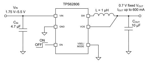
Figure 9-52. TPS62806 VSEL Connected to GND for 0.7-V Fixed  $V_{OUT}$
