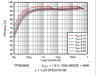
Figure 9-13. Efficiency Power Save Mode  $V_{OUT} = 1.8 V$
