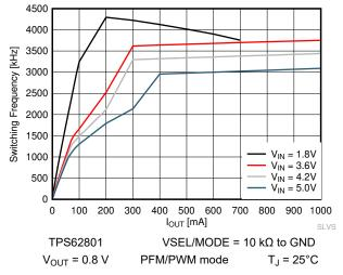
Figure 9-23. Switching Frequency vs Output Current
