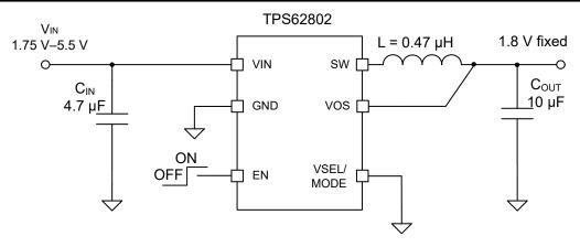
Figure 9-50. TPS62802 VSEL Connected to GND for 1.8-V Fixed V<sub>OUT</sub>
