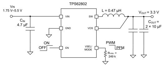
Figure 9-49. TPS62802 Adjustable 3.3-V V<sub>OUT</sub> Application Circuit
