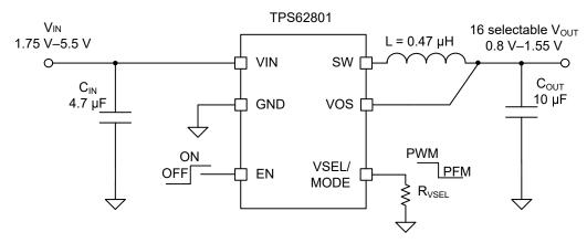
Figure 9-1. TPS62801 Adjustable V<sub>OUT</sub> Application Circuit
