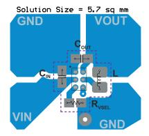
Figure 11-1. PCB Layout Example
