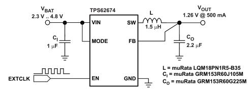
Figure 50. 1.26V CMOS Sensor Embedded Power Solution — Featuring Sub 0.4mm Profile
