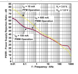
Figure 18. PSRR vs Frequency
