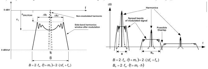
Figure 26. Spectrum of a Frequency Modulated Sin. Wave with Sinusoidal Variation in Time
