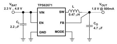
Figure 28. 1.8V/0.5A Power Supply Using TPS62671
