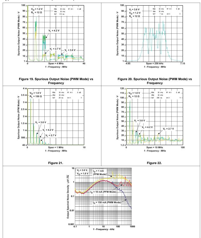
Figure 23. Output Spectral Noise Density vs Frequency
