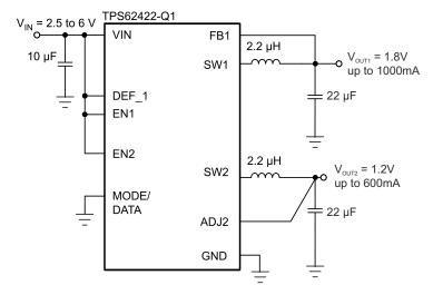
Figure 9-24. TPS62422-Q1 Fixed 1.8-V and 1.2-V Outputs
