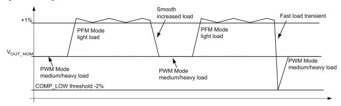
Figure 8-1. Dynamic Voltage Positioning
