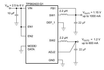
Figure 9-23. TPS62422-Q1 Fixed 1.15-V and 1.2-V Outputs
