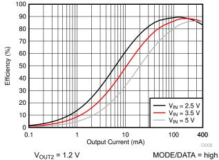
Figure 9-8. TPS62406-Q1 Efficiency, V<sub>OUT2</sub>
