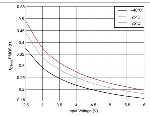
Figure 7-4. r<sub>DS(on)</sub> PMOS vs V<sub>IN</sub>
