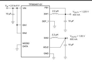
Figure 9-22. TPS62407-Q1 Fixed 1.225-V and 1.85-V Outputs
