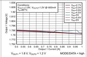
Figure 9-10. TPS62422-Q1 V<sub>OUT1</sub> vs. I<sub>OUT1</sub>
