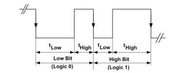
Figure 8-6. EasyScale - Bit Coding
