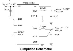
applications such as Advanced Driver Assistance Systems (ADAS). They provide two independent output voltage rails powered by a standard 3.3-V or 5-V voltage rail, with fixed output voltages optimized for powering the CMOS imager or serializer-deserializer in ADAS camera modules.
