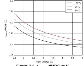
Figure 7-5. r<sub>DS(on)</sub> NMOS vs V<sub>IN</sub>
