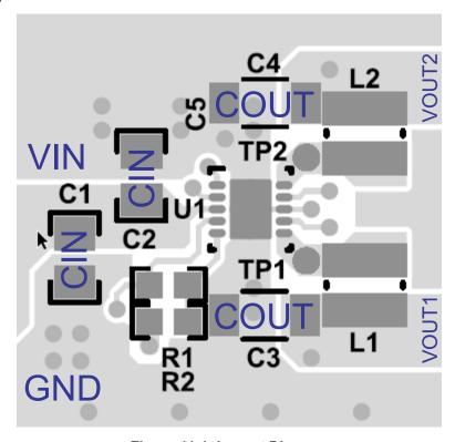
Figure 11-1. Layout Diagram
