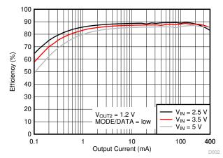
TPS62406-Q1 Efficiency vs Output Current, V<sub>OUT2</sub>
