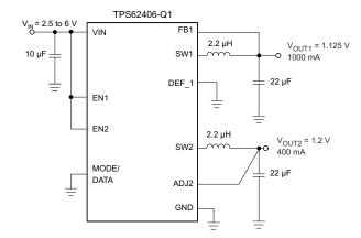
Figure 9-21. TPS62406-Q1 Fixed 1.125-V and 1.2-V Outputs
