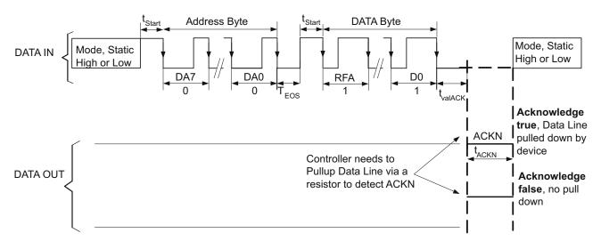
Figure 8-5. EasyScale Protocol Including Acknowledge
