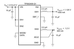
Figure 9-1. Typical Application Schematic
