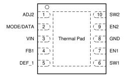
Figure 6-1. DRC Package 10-Pin VSON With Thermal Pad Top View
