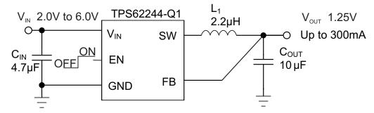
Figure 6. TPS62244Q1, Fixed 1.25 V V<sub>OUT</sub>
