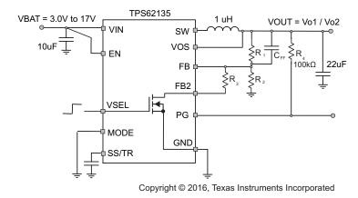
Figure 83. Typical Application using VSEL
