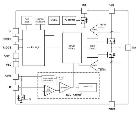
The discharge switch on the VOS pin is only available in the TPS62135.
