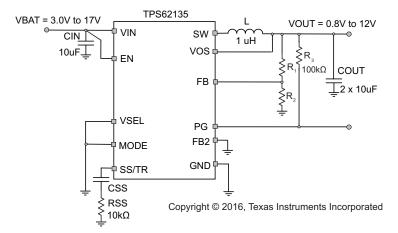
Figure 90. Adding a Series Resistor to CSS
