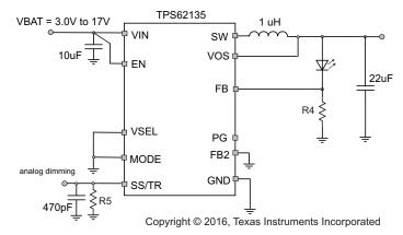
Figure 86. Single Power LED Supply
