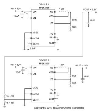
Figure 4. Schematic for Ratiometric and Simultaneous Startup
