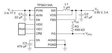
Figure 4. TPS62134A Typical Application
