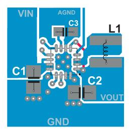
Figure 19. TPS62134x Layout Example
