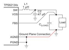
Figure 3. Remote Sense Connection
