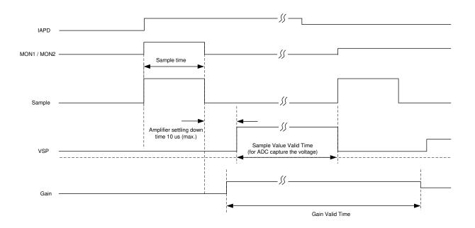
Figure 11. TPS61390 Sample / Hold Circuit Timing
