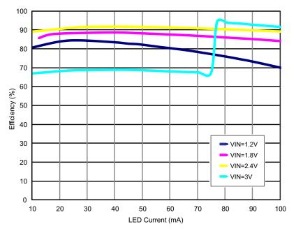
Figure 24. LED Driver Efficiency
