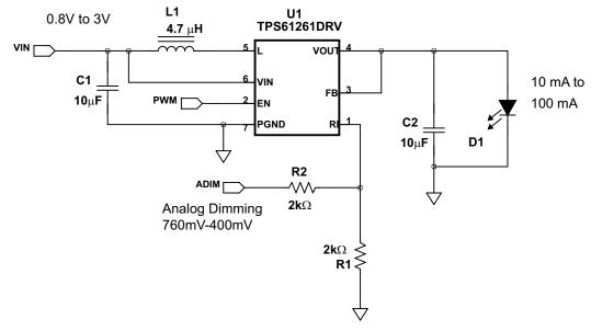
Figure 23. TPS61260 LED Driver Application Circuit
