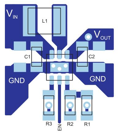
Figure 25. PCB Layout Suggestion
