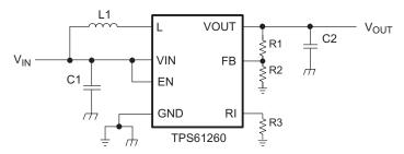
Figure 18. TPS61260 Typical Application Circuit
