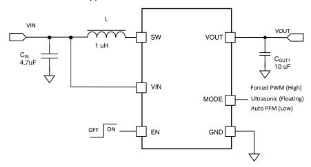
Figure 9-10. Typical Application with Minimum Output Capacitance
