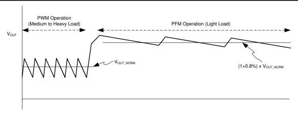
Figure 8-3. Output Voltage in Auto PFM / PWM Mode
