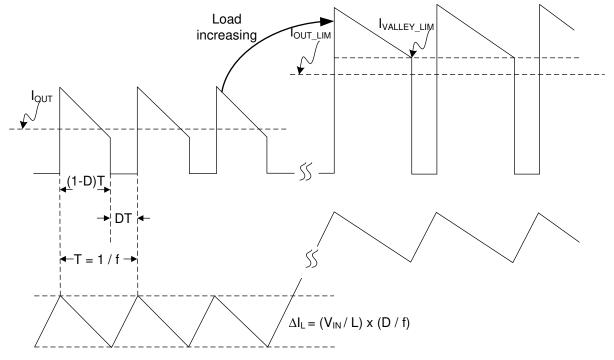
Figure 8-1. Current Limit Operation
