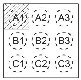
Figure 6-1. 9-Pin DSBGA YFF Package (Top View)
