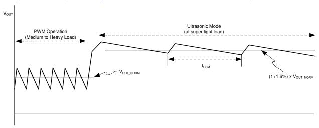
Figure 8-4. Ultrasonic Mode Operation
