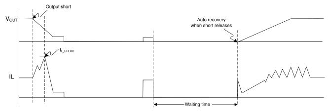
Figure 8-2. Hiccup Mode Short Protection
