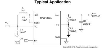
The typical operating frequency is 1.15 MHz, which allows the use of small inductor and capacitors to achieve a small solution size. The TPS61230A provides an adjustable output voltage via an external resistor divider.
