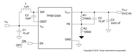
Figure 25. TPS61230A 5-V Output with Cff Typical Application
