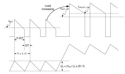
Figure 13. Current Limit Operation
