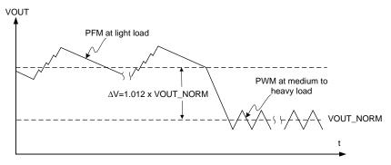
Figure 14. Output Voltage in PFM / PWM Mode
