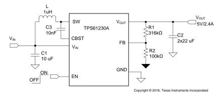
Figure 15. TPS61230A 5-V Output Typical Application
