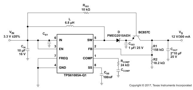
Figure 17. Typical Application With External Load Disconnect Switch
