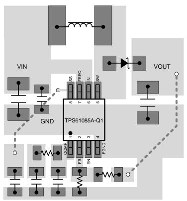
Figure 22. TPS61085A-Q1 Layout Example
