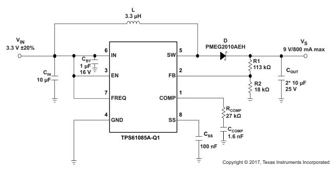
Figure 15. Typical Application, 3.3 V to 9 V (f<sub>sw</sub> = 1.2 MHz)
