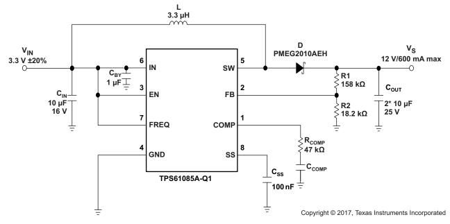
Figure 8. Typical Application, 3.3 V to 12 V (f<sub>sw</sub> = 1.2 MHz)
