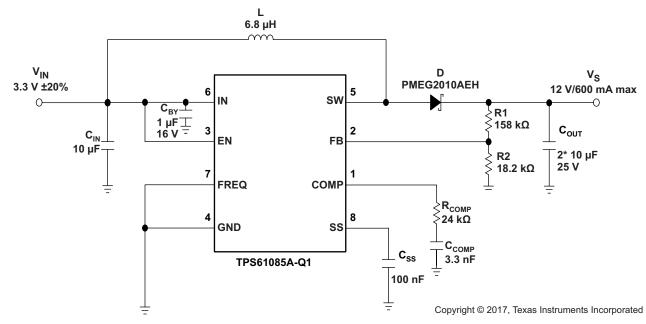
Figure 14. Typical Application, 3.3 V to 12 V (f<sub>sw</sub> = 650 kHz)
