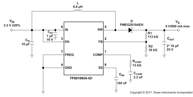
Figure 16. Typical Application, 3.3 V to 9 V (f<sub>sw</sub> = 650 kHz)
