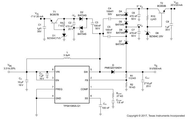
Figure 18. Typical Application 3.3 V to 9 V (f<sub>sw</sub> = 1.2 MHz) For TFT LCD With External Charge Pumps (VGH, VGL)
