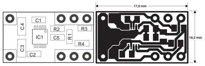
Figure 24. Recommended Component Placement and Board Layout
