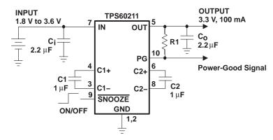
Figure 23. Typical Operating Circuit TPS60211 With Power-Good Comparator
