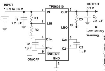
Figure 1. Typical Application Circuit With Low-Battery Warning
