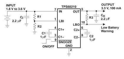
Figure 21. Typical Operating Circuit TPS60210 With Low-Battery Comparator
