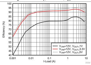
Figure 15. Efficiency, FCCM, F<sub>SW</sub> = 600 kHz
