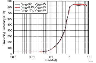
Figure 23. F<sub>SW</sub> Load Regulation, Eco-mode, F<sub>SW</sub> = 800 kHz
