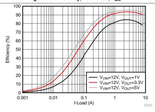
Figure 17. Efficiency, OOA-mode,  $F_{SW} = 1 \text{ MHz}$
