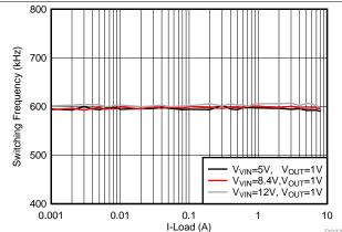
Figure 21.  $F_{SW}$  Load Regulation, OOA-mode,  $F_{SW}$  = 600 kHz
