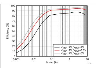
Figure 13. Efficiency, Eco-mode, F<sub>SW</sub> = 600 kHz
