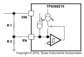
Figure 22. Adjustable VIN Under Voltage Lock Out
