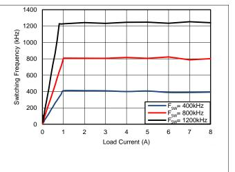
Figure 20.  $F_{SW}$  Load Regulation, Mode = DCM,  $V_{IN}$  = 12V,  $V_{OUT}$ =1.2V
