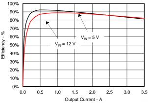
Figure 3. 1.8-V Efficiency
