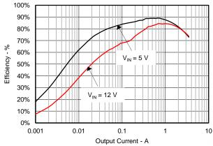
Figure 2. 1-V Efficiency, Eco-mode™
