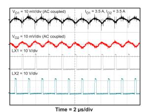
Figure 12. Output Ripple at 3.5 A, Forced PWM
