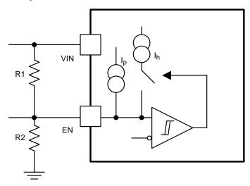
Figure 25. Adjustable VIN Under-Voltage Lockout
