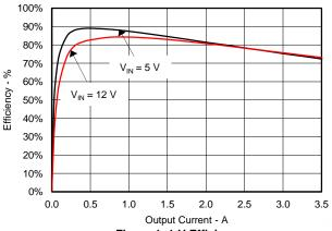
Figure 1. 1-V Efficiency
