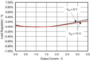
Figure 8. 1.8-V Load Regulation, Eco-mode
