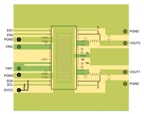
Figure 33. TPS563900 Layout on 2-layer PCB
