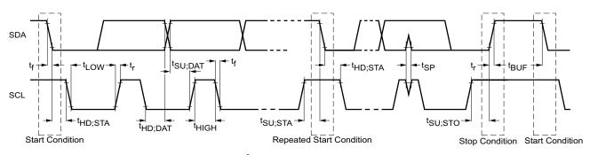
Figure 28. I<sup>2</sup>C Interface Timing Diagram
