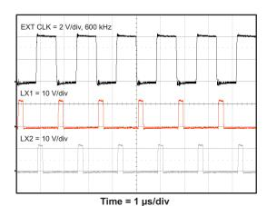
Figure 23. Synchronization at 600 kHz
