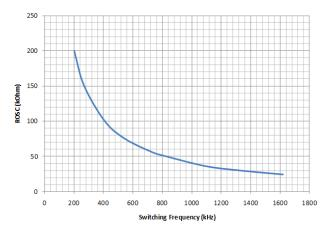
Figure 26. ROSC Versus Switching Frequency
