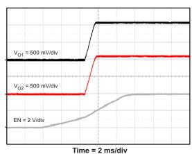
Figure 14. Startup With Enable
