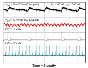
Figure 13. Output Ripple, Buck1 at 0.05 A, Buck 2 at 0.3 A Auto PSM-PWM Mode
