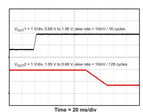
Figure 22. Voltage Change With I<sup>2</sup>C Control
