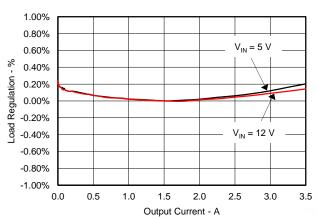
Figure 6. 1-V Load Regulation, Eco-mode
