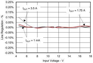
Figure 9. Line Regulation,  $V_{OUT}1 = 1.0 V$ , Eco-mode = OFF
