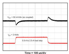
Figure 16. Load Transient, Buck 1 (0.5 A to 2.5 A)
