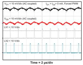
Figure 11. Output Ripple at 0 A, Forced PWM
