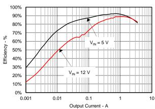
Figure 4. 1.8-V Efficiency, Eco-mode
