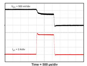
Figure 18. Overcurrent Protection, Buck 1
