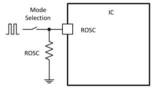
Figure 27. Resistor Mode and Synchronization Mode
