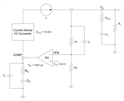
Figure 32. DC-DC Loop Compensation
