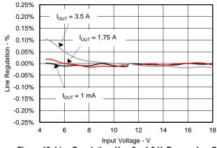
Figure 10. Line Regulation, V<sub>OUT</sub>2 = 1.0 V, Eco-mode = OFF
