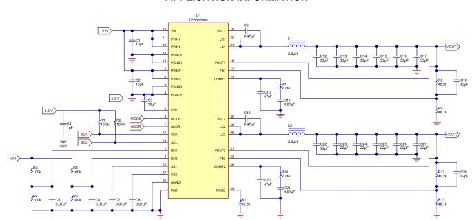
Figure 31. 1.1-V Output TPS563900 Design Example
