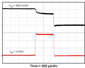
Figure 20. Overcurrent Protection, Buck 2
