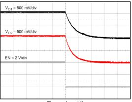
Time = 1 ms/div Figure 15. Shutdown With Enable
