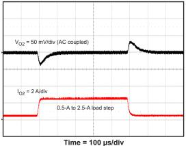
Figure 17. Load Transient, Buck 2 (0.5 A to 2.5 A)
