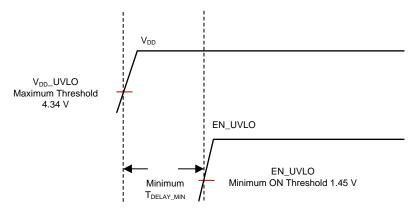
Figure 16. Minimum Delay Between V<sub>DD</sub> and EN\_UVLO to Support the Use of 4-ms and 8-ms SS settings
