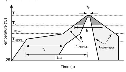
Figure 32. Recommended Reflow Oven Thermal Profile
