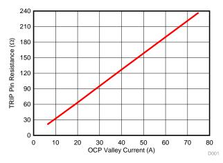
Figure 14. Current Limit Resistance vs OCP Valley Overcurrent Limit
