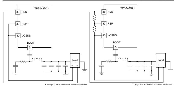
Figure 17. Remote Sensing Without Feedback Resistors
