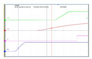
Figure 15. Proper Sequencing of  $V_{\text{DD}}$  and EN\_UVLO to Support the Use of 4-ms SS Setting
