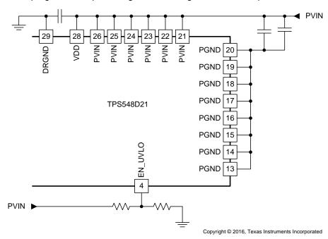
Figure 13. Programming the UVLO Voltage
