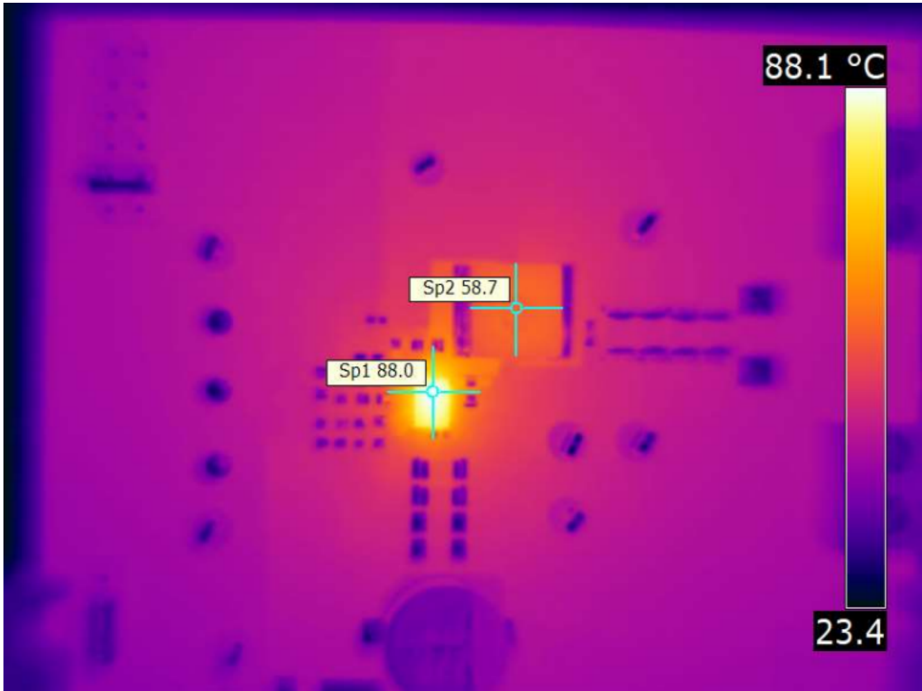
Figure 10-2. Thermal Image At 25°C Ambient
