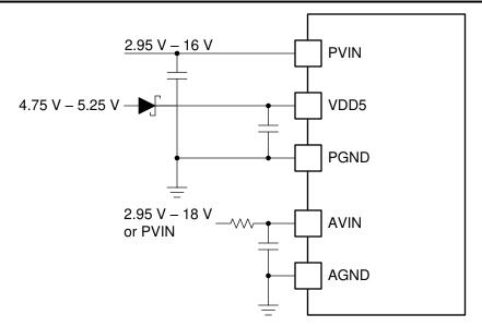
Figure 7-4. TPS546D24A Separate PVIN, AVIN, and VDD5 Connections
