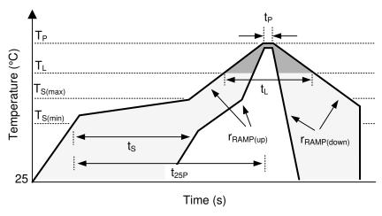
Figure 10-2. Recommended Reflow-Oven Thermal Profile
