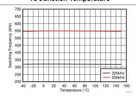
Figure 6-16. Switching Frequency vs Junction Temperature
