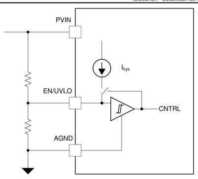
Figure 7-5. TPS546D24A UVLO Voltage Divider
