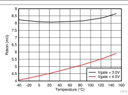
Figure 6-14. High-Side MOSFET On-Resistance (R DS(on))
