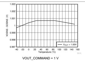
Figure 6-15. Output Voltage vs Junction Temperature
