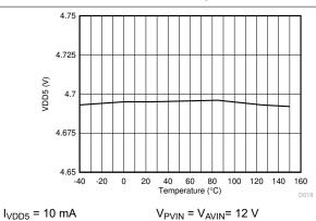
Figure 6-18. VDD5 Voltage vs Junction Temperature
