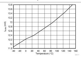
Figure 6-17. Non-Switching Input Current (I<sub>AVIN</sub>) vs Junction Temperature
