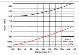
Figure 6-13. Low-Side MOSFET On-Resistance (R DS(on))
