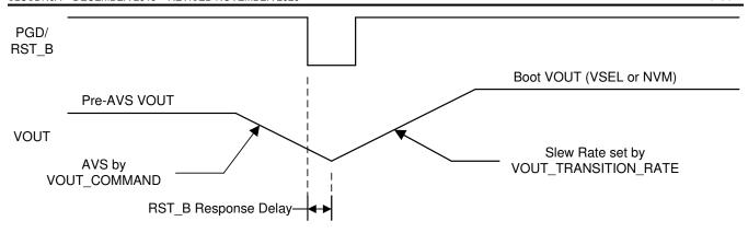
Figure 7-7. TPS546D24A Output Voltage Reset
