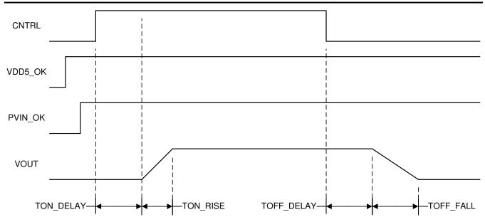
Figure 7-6. TPS546D24A Start-up and Shutdown
