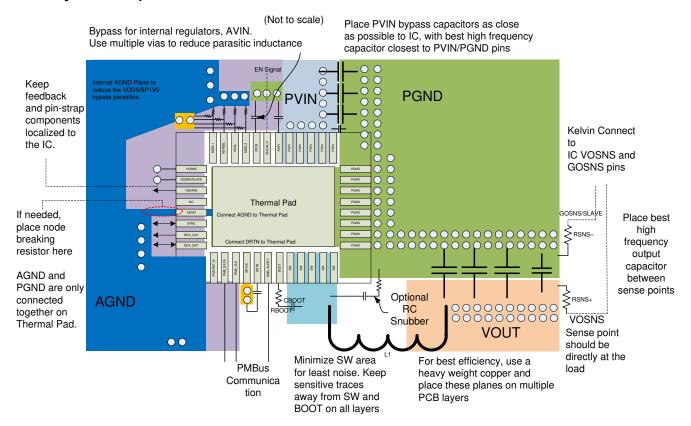
Figure 10-1. PCB Layout Recommendation
