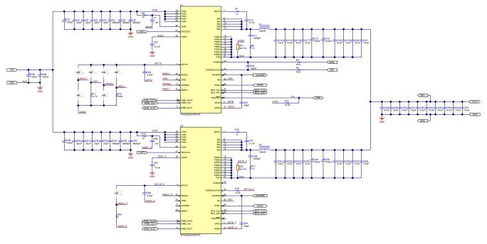
Figure 8-11. TPS546D24A Two-Phase Application
