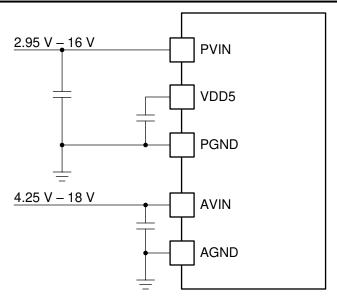
Figure 7-2. TPS546D24A Separate PVIN and AVIN connections
