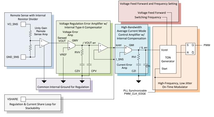
Figure 7-1. Average Current Mode Control Block Diagram
