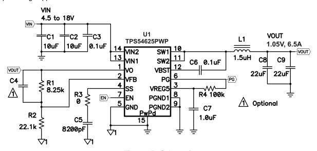
Figure 15. Schematic
