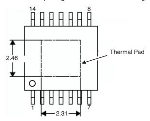
Figure 16. Thermal Pad Dimensions
