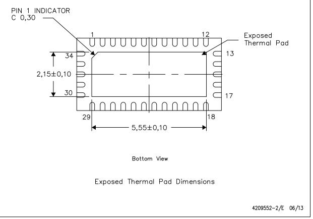
NOTE: All linear dimensions are in millimeters
