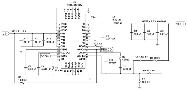
Analog and power grounds are ties at the pad under the package of the IC
