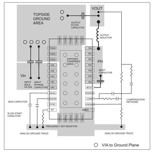
Figure 11. TPS54617 PCB Layout
