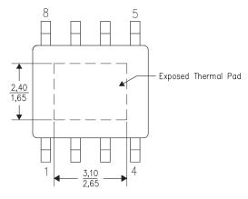
Figure 16. Thermal Pad Dimensions (Top View)
