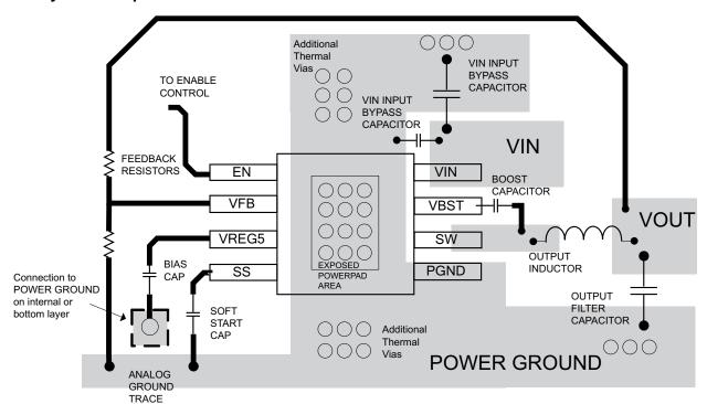
Figure 20. TPS54428 Layout for the DDA Package
