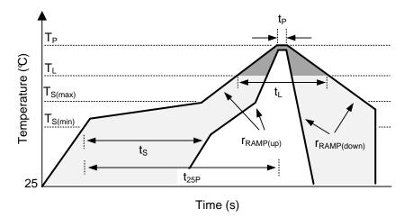
Figure 47. Recommended Reflow Oven Thermal Profile
