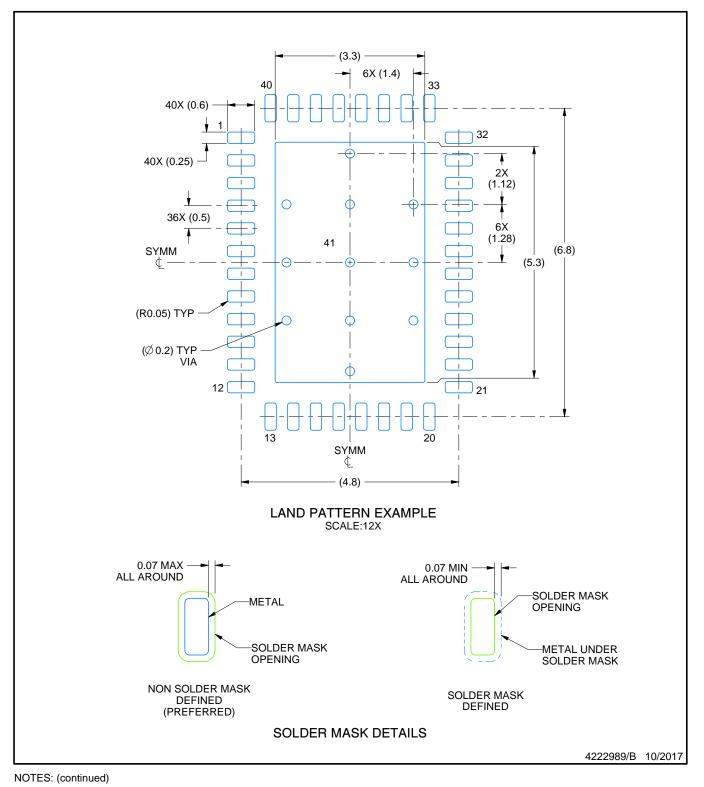
5. This package is designed to be soldered to a thermal pad on the board. For more information, see Texas Instruments literature number SLUA271 (www.ti.com/lit/slua271).
