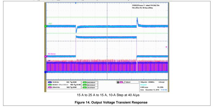
VIN = VDD = 12 V,  $T_A = 25^{\circ}C$ ,  $R_{RT} = 40.2 \text{ k}\Omega$ ,  $T_A = 25^{\circ}C$  (unless otherwise specified)
