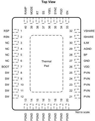
RVF Package 40-Pin LQFN-CLIP With Thermal Pad Top View
