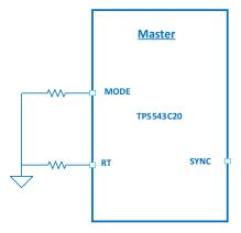
Figure 16. Standalone: RT Pin Sets the Switching Frequency
