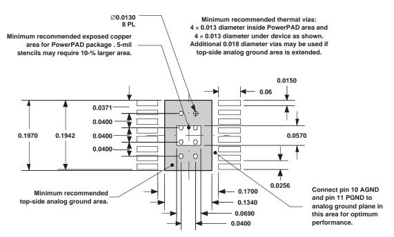
Figure 24. Thermal Considerations for PowerPAD™ Layout
