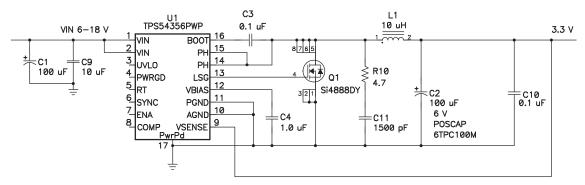
Figure 28. 3.3-V Power Supply With Sanyo POSCAP Output Filter Capacitor
