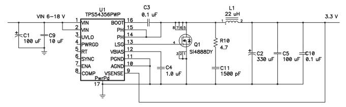
Figure 25. Application Circuit, 12 V to 3.3 V
