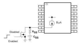
Figure 2. Interfacing to the ENA Pin
