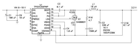
Figure 30. 3.3-V Power Supply With Sanyo OSCON Output Filter Capacitor
