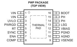
NOTE: If there is not a pin 1 indicator, turn device to enable reading the symbol from left to right. Pin 1 is at the lower left corner of the device.
