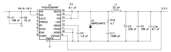
Figure 26. Power Supply With Schottky Diode
