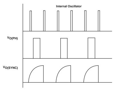
Figure 4. SYNC Output Waveform
