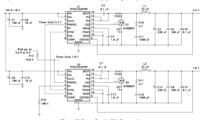
Figure 27. Power Supply With Sequencing
