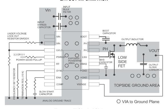
Figure 23. TPS5435x PCB Layout
