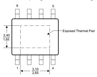
Figure 17. Thermal Pad Dimensions
