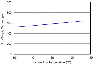
Figure 1. VIN CURRENT vs JUNCTION TEMPERATURE
