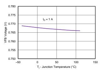
Figure 12. VFB VOLTAGE vs JUNCTION TEMPERATURE (I<sub>O</sub> = 1 A)
