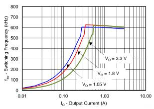
Figure 11. SWITCHING FREQUENCY vs OUTPUT CURRENT
