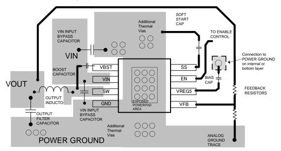
Figure 18. PCB Layout
