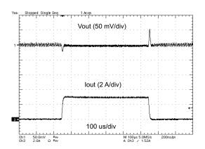
Figure 6. 1.05-V, LOAD TRANSIENT RESPONSE
