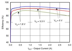
Figure 8. EFFICIENCY vs OUTPUT CURRENT
