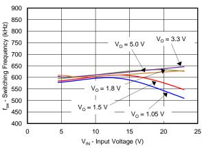
Figure 10. SWITCHING FREQUENCY vs INPUT VOLTAGE ( $I_0 = 1 \text{ A}$ )
