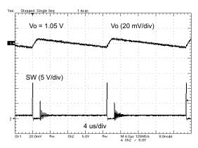
Figure 13. VOLTAGE RIPPLE AT OUTPUT ( $I_0 = 3A$ )
