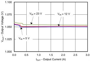
Figure 4. 1.05-V OUTPUT VOLTAGE vs OUTPUT CURRENT
