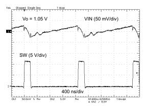
Figure 15. VOLTAGE RIPPLE AT INPUT ( $I_0 = 3 A$ )
