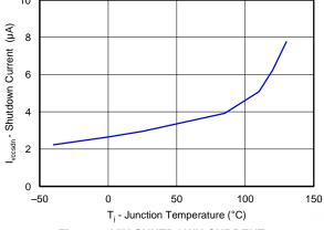
Figure 2. VIN SHUTDOWN CURRENT vs JUNCTION TEMPERATURE
