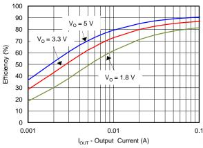
Figure 9. LIGHT LOAD EFFICIENCY vs OUTPUT CURRENT
