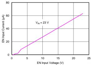
Figure 3. EN CURRENT vs EN VOLTAGE
