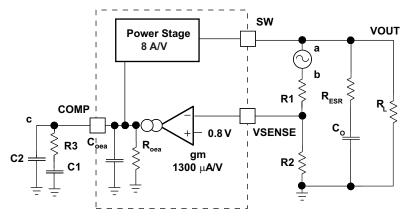
Figure 14. Small Signal Model for Loop Response
