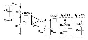
Figure 17. Types of Frequency Compensation
