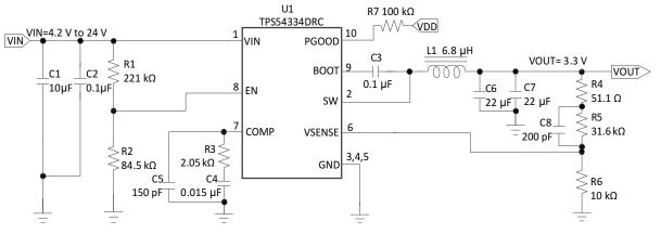
Figure 18. Typical Application Schematic, TPS54334
