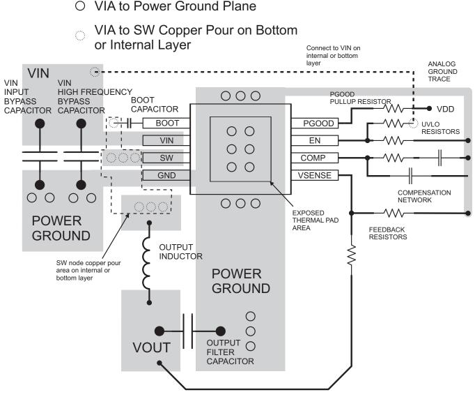
Figure 34. TPS54334DDA Board Layout
