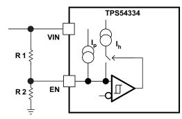
Figure 13. Adjustable VIN Undervoltage Lockout
