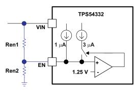
Figure 11. Adjustable Input Undervoltage Lockout
