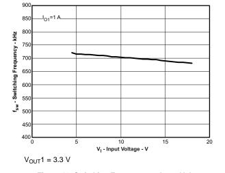
Figure 12. Switching Frequency vs Input Voltage
