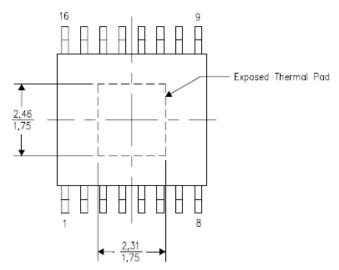
Figure 27. Thermal Pad Dimensions
