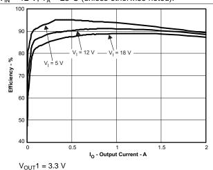
Figure 8. Efficiency vs Output Current
