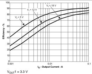
Figure 9. Efficiency vs Output Current
