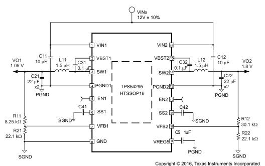
Figure 16. Schematic Diagram for the Design Example
