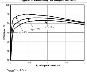
Figure 10. Efficiency vs Output Current
