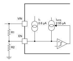
Figure 24. Adjustable Undervoltage Lockout
