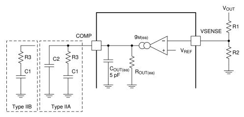
Figure 34. Types of Frequency Compensation
