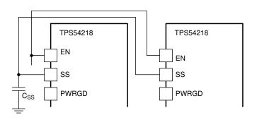
Figure 26. Sequential Start-up using EN and PWRGD
