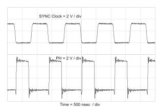
Figure 29. Synchronizing to a System Clock
