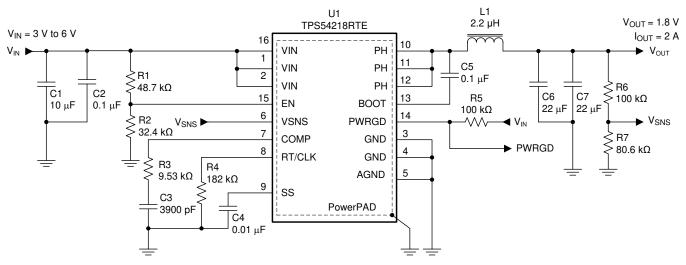
Figure 35. Typical Application Schematic, TPS54218
