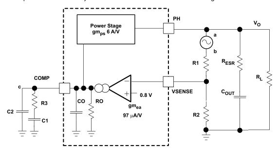
Figure 45. Small-Signal Model for Loop Response
