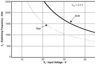
Figure 40. Maximum Switching Frequency vs. Input Voltage
