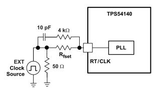
Figure 41. Synchronizing to a System Clock
