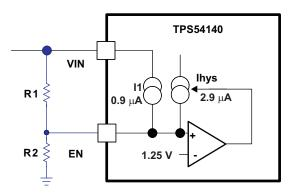
Figure 27. Adjustable Undervoltage Lockout (UVLO)
