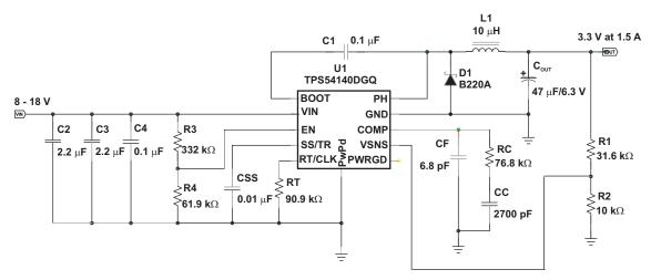
Figure 50. High Frequency, 3.3-V Output Power Supply Design With Adjusted UVLO
