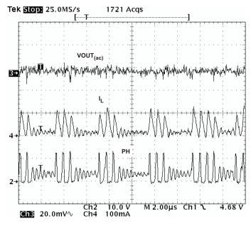
Figure 49. Pulse-Skip Mode Operation
