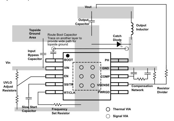
Figure 64. PCB Layout Example
