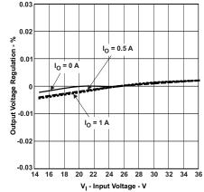
Figure 23. Output Voltage Regulation % vs. Input Voltage
