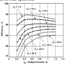
Figure 21. Efficiency vs. Output Current
