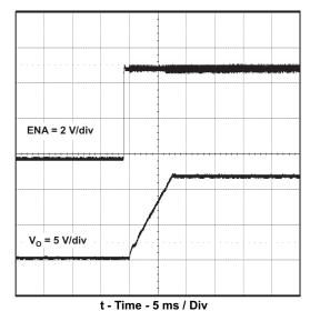
Figure 20. Startup Waveform, ENA and Vo
