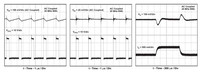
Figure 24. Input Voltage Ripple and PH Node,  $I_0 = 1$  A
