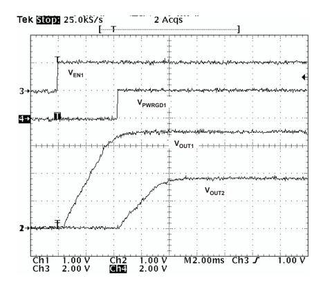
Figure 30. Sequential Start-Up Using EN and PWRGD
