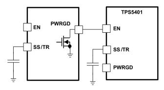
Figure 29. Schematic for Sequential Start-Up Sequence
