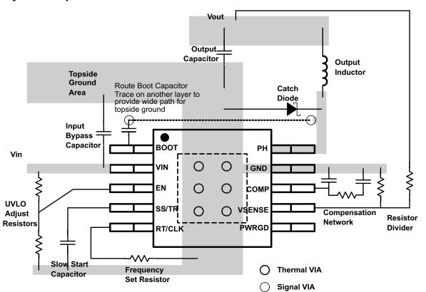
Figure 54. PCB Layout Example
