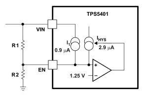
Figure 27. Adjustable Undervoltage Lockout (UVLO)
