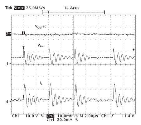
Figure 39. Pulse-Skip Mode Operation
