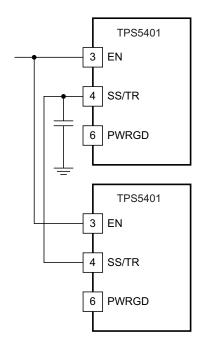
Figure 31. Schematic for Ratiometric Start-Up Sequence
