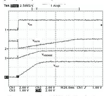
Figure 28. Operation of SS/TR Pin When Starting
