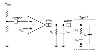
Figure 41. The Compensation Recommended for the TPS5401
