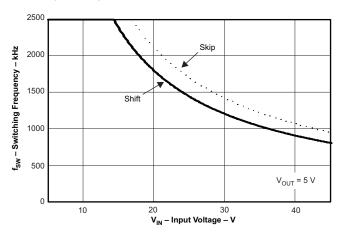
Figure 37. Maximum Switching Frequency vs. Input Voltage
