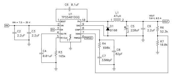
Figure 40. Typical Application Schematic
