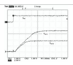
Figure 34. Ratiometric Start-Up With V<sub>OUT2</sub> Leading V<sub>OUT1</sub>
