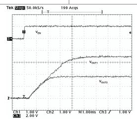
Figure 36. Simultaneous Start-Up
