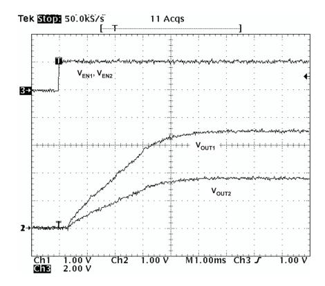
Figure 32. Ratiometric Start-Up Using Coupled SS/TR Pins
