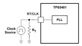
Figure 38. Synchronizing to a System Clock
