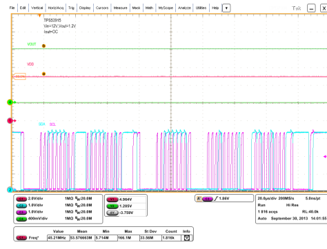
Figure 32. I 2 C READ (Address=31d, Cmd=0x79): ACK 0x10C8. IO C = 15 A
