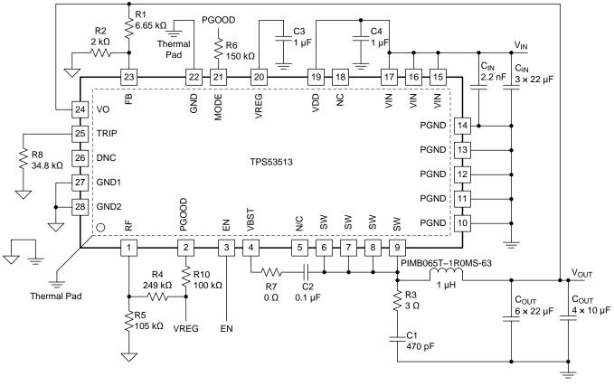
Figure 43. Application Circuit Diagram
