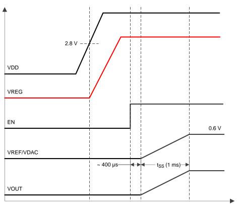
Figure 33. Power-up Sequence Waveforms
