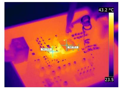
$T_{A} = 23^{\circ}C, \ f_{SW} = 500 \ \text{kHz}, \ V_{IN} = 12 \ \text{V}, \ V_{OUT} = 1.24 \ \text{V}, \ I_{OUT} = 8 \ \text{A}, \ R_{BOOT} = 0 \ \Omega, \ \text{SNB} = 3 \ \Omega + 470 \ \text{pF}$ Inductor: L<sub>OUT</sub> = 1 µH, PIMB103T-1R0MS-63, 10 mm × 11.2 mm × 3 mm, 5.3 mΩ
