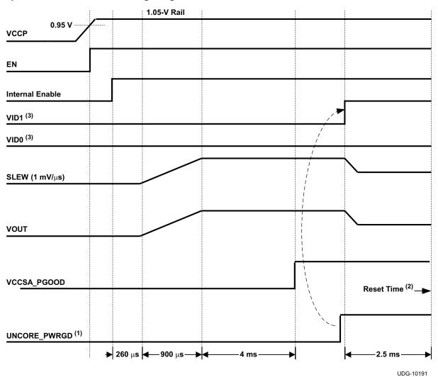
Figure 6. Fixed VID/Fixed Step Startup and VID Toggle Timing Diagram for 2011 Intel Platform
