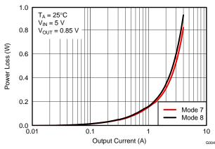
Figure 11. Power Loss vs. Output Current
