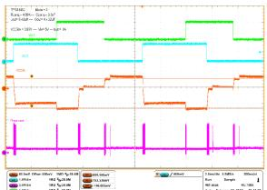
Figure 14. Mode=8, I<sub>OUT</sub> = 0 A, VID Transitioning
