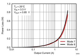
Figure 10. Power Loss vs. Output Current
