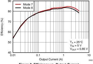
Figure 9. Efficiency vs. Output Current
