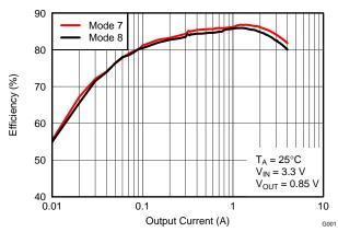
Figure 8. Efficiency vs. Output Current
