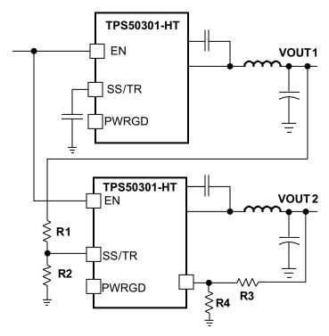
Figure 24. Ratiometric and Simultaneous Start-Up Sequence
