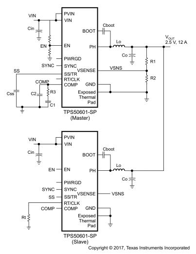
Figure 30. Parallel Configuration Showing Master and Slave
