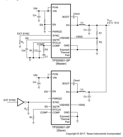
Figure 31. Parallel Configuration With External Sync
