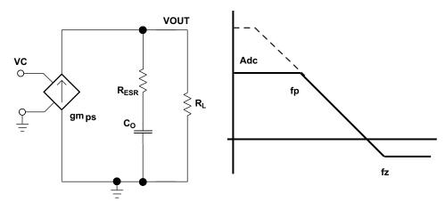
Figure 27. Simplified Frequency Response for Peak Current Mode Control
