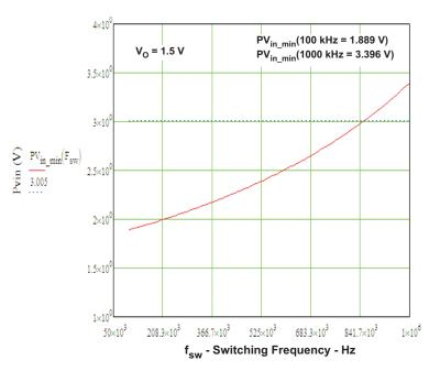
Figure 17. PV<sub>IN</sub> vs Frequency
