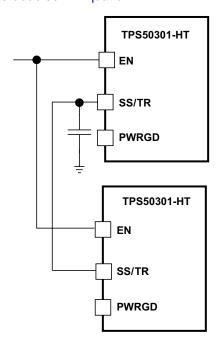
Figure 23. Ratiometric Start-Up Sequence
