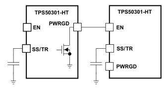
Figure 22. Sequential Start-Up Sequence
