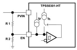
Figure 18. Adjustable VIN UVLO
