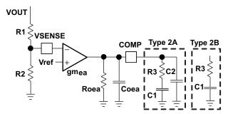
Figure 28. Types of Frequency Compensation
