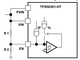
Figure 20. Adjustable VIN and PVIN UVLO
