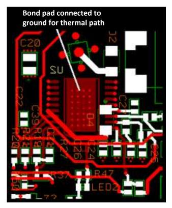
Figure 33. PCB Layout Example
