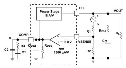
Figure 25. Small Signal Model For Loop Response
