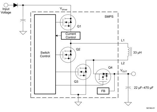
Figure 19. Buck/Boost Switch Mode Configuration
