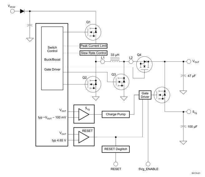
Figure 18. Current-Limit Switched Output 5Vg
