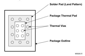
Figure 22. Package and PCB Land Configuration for a Multilayer PCB
