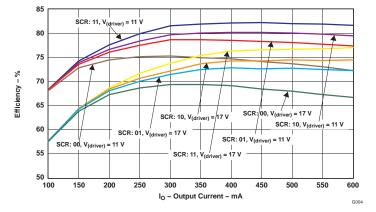
NOTE: The average converter efficiency with four different slew rate controls (SCRx) on the Q1 switching FET with input voltage V<sub>(driver)</sub> = 11 V and 17 V, T<sub>A</sub> = 125°C.
