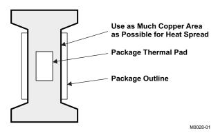
Figure 24. Land Configuration for Single-Layer PCB
