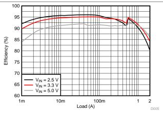
Figure 7. 1.8-V Output Efficiency
