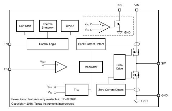
Figure 4. TLV62569 Functional Block Diagram
