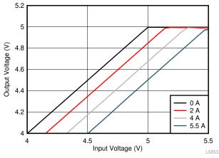
Figure 8-10. Overall Dropout Characteristics (V<sub>OUT</sub> = 5 V)
