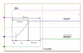
Figure 8-4. Typical Start-Up Waveform
