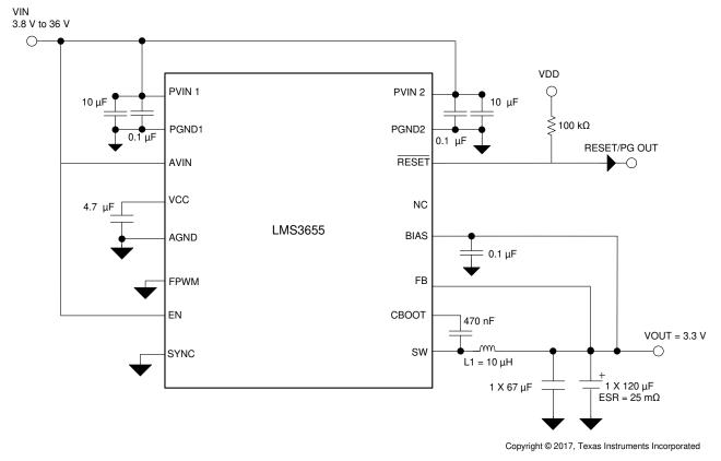
Figure 9-16. Fixed 3.3-V, 5.5-A Output Power Supply
