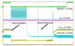
Figure 8-5. Short-Circuit Transient and Recovery
