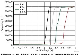
Figure 8-11. Frequency Dropout Characteristics (V<sub>OUT</sub> = 5 V)
