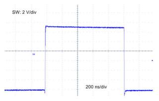
Figure 8-1. Switch Node Waveform (V<sub>IN</sub> = 13.5 V, I<sub>OUT</sub> = 5.5 A)
