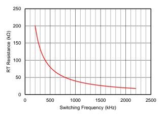
Figure 14. RT vs Frequency Curve
