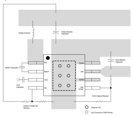
Figure 34. SOIC Layout
