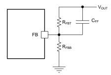
Figure 22. Feedforward Capacitor for Loop Compensation
