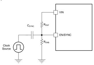
Figure 17. Synchronize to External Clock
