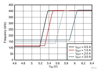
Figure 20. Frequency Foldback at Dropout ( $V_{OUT} = 5 \text{ V}$ ,  $f_{SW} = 400 \text{ kHz}$ )
