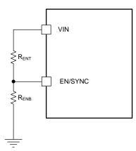
Figure 16. System UVLO by Enable Divider
