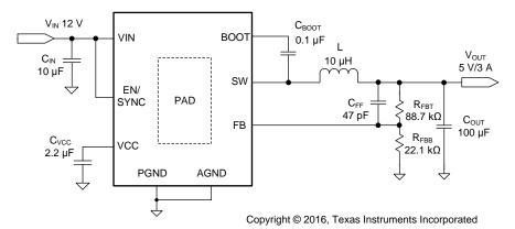
Figure 23. Application Circuit
