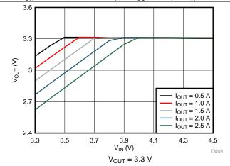
Figure 7. Dropout Curve
