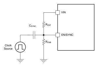
Figure 16. Synchronize to External Clock
