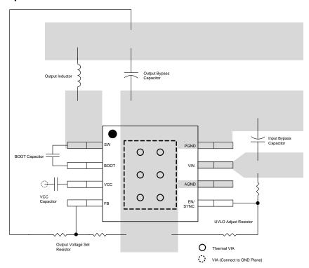
Figure 33. SOIC Layout
