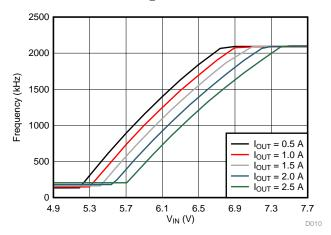
Figure 19. Frequency Foldback at Dropout (V<sub>OUT</sub> = 5 V, f<sub>SW</sub> = 2100 kHz)
