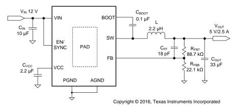
Figure 22. LMR23625-Q1 Application Circuit
