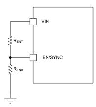
Figure 15. System UVLO by Enable Divider
