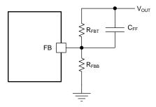
Figure 21. Feed-forward Capacitor for Loop Compensation
