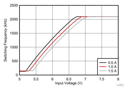
Figure 20. Frequency Foldback at Dropout (V<sub>OUT</sub> = 5 V, f<sub>SW</sub> = 2100 kHz)
