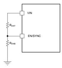
Figure 16. System UVLO by Enable Divider
