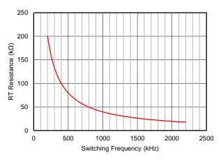
Figure 14. RT vs Frequency Curve
