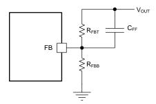
Figure 21. Feedforward Capacitor for Loop Compensation
