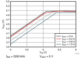
Figure 7. Dropout Curve
