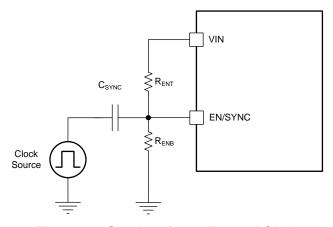
Figure 17. Synchronize to External Clock
